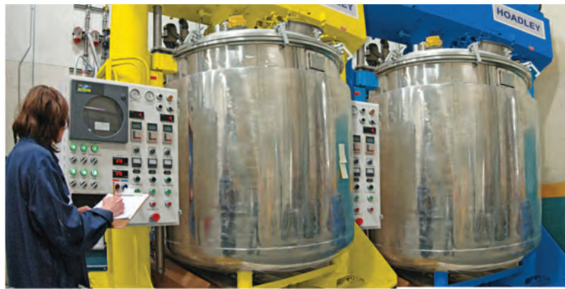
The Smooth-On factory houses two of the largest silicone mixing vessels in North America (1,500 gallons / 5,678 liters), each powered by 3 x 100 horse power motors and high-shear mixing blades.
